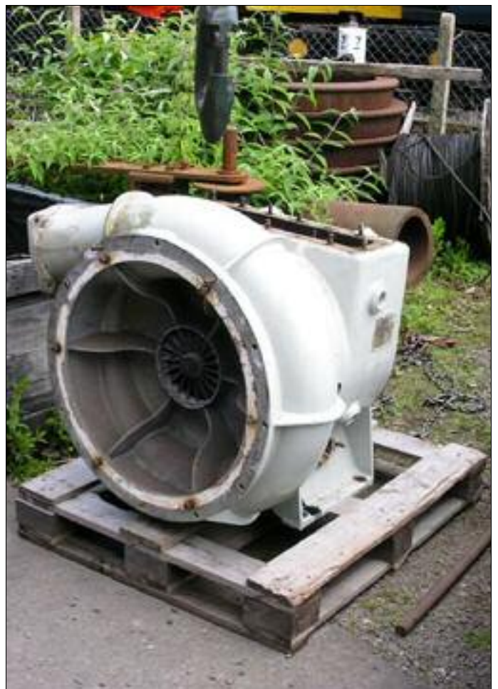
33 002's turbo has been craned out of the loco and dispatched for assessment / overhaul to a company near Barrow Hill Pete Burrow
