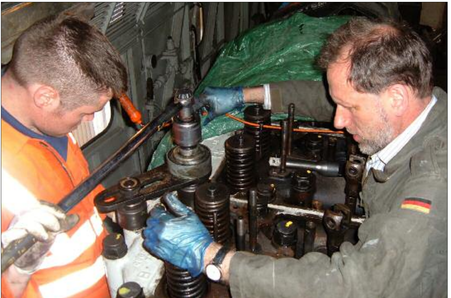
Jon and Robin torquing down 33 002's cylinder heads to 750lb/ft. The torque multiplier makes this a bit easier
