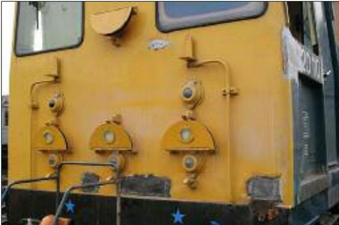
20 110 receiving cab corrosion repairs October 2007. Pete Burrow
