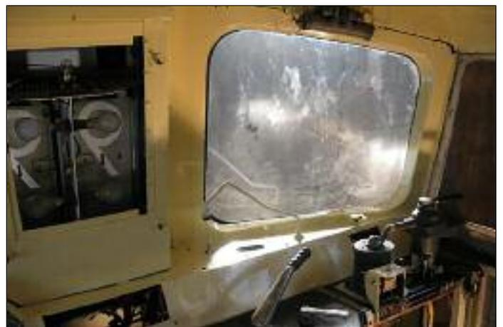
33 002's cab refurbishment in progress. Painting is now advanced and at the glossing stage in the original cream colour scheme. No 2 Cab is seen above at the end of January showing the extent of progress to date. No 1 Cab is not far behind No 2 Cab. Neil and Pete have been overhauling items from the cabs off site. The horn valves and sanders have also been freed off.
